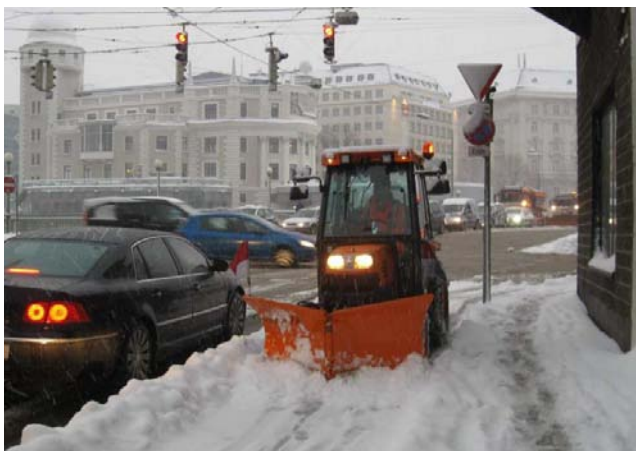
Small snow removal vehicle clearing a buffered bike lane in Vienna, Austria. Photo Credit: http://www.ibikeoulu.com/presentations/presentation_oulu_szeiler_130213.pdf
