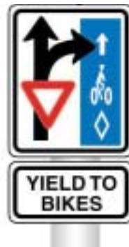
This sign may be used where a travel lane crosses a colored-lane treatment
