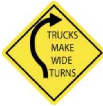
Trucks Make Wide Turns Sign: Indicates to bicyclists and motorists that large trucks will swing left prior to making right turn. Sign warns bicyclists of potential right side conflicts.
