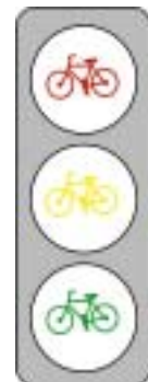
This bicycle-signal head may be used as per the standards set by CTCDC, 11/19/99. The signal provides a separate phase specifically for bicyclists.
