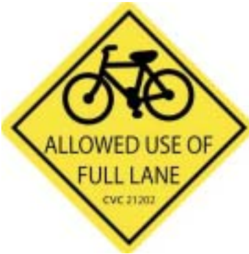
Bicycles Allowed Full Use of Lane Sign: Indicates bicycles allowed full use of lane in situations where no bicycle lanes exist or where merging with vehicle traffic is required for safe operations.
